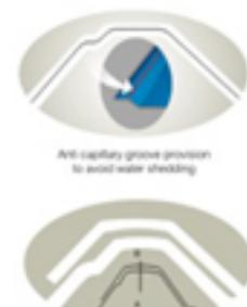
Provision of reverse leg facilitates unique lapping which ensures proper covering at the bottom side lap.
